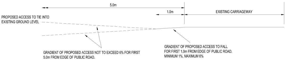
WHERE EXISTING GRADIENT EXCEEDS 6%, ACCESS TO FALL FOR FIRST 1.0m (MIN 1%, MAX 6%), THEN TIE INTO EXISTING GROUND LEVEL AS SPECIFIED ON INDIVIDUAL ACCESS DRAWINGS.
